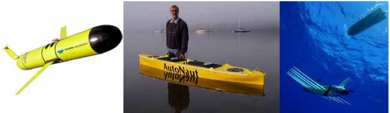
From left to right, the Slocum G2 Glider (longest endurance UUV from data set); AutoNaut from MOST (Autonomous Vessels), Ltd. (the longest endurance USV); Wave Glider SV3 from Boeing/Liquid Robotics (a hybrid USV/UUV with endurance of multiple years).
