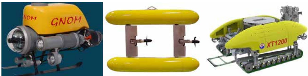
From left to right, GNOM Standard from Indel-Partner Ltd. (the smallest ROV from the data set); SQX-500 from Marpot (a unique hydrodynamic dual hull design
